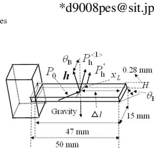
Fig. 2. Geometry of X-rays and the sample.
