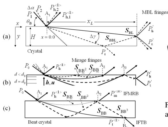
Fig. 1. Beam geometries in a perfect crystal when it is unbent (a), and it is bent (b, c).
