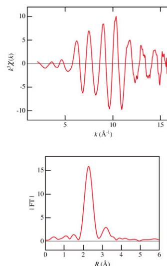
Figure 1. In K XAFS signal (upper) and its Fourier-transform (lower) of TlInSe<sub>2</sub> measured at room temperature.
