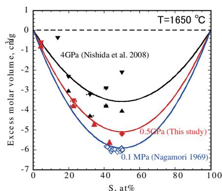
Fig. 3 The excess molar volume of liquid Fe-S as a function of Sulfur content.
