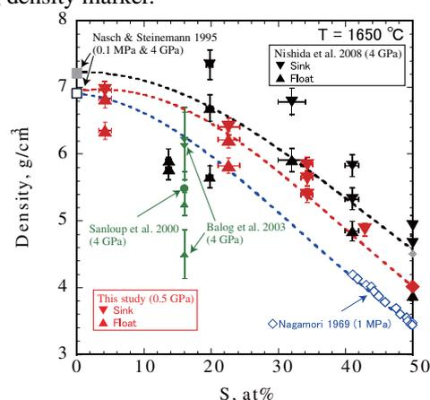
Fig. 2 Density of liquid Fe-S as a function of sulfur content.
