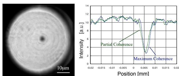
Fig.3 Blur-corrected image (latex particle of  $8\mu\text{m}$ ) observed at the SPring-8.
