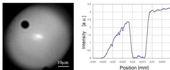
Fig.1 Blur-corrected image (latex particle of  $8\mu\text{m}$ ) observed at the Photon Factory.
