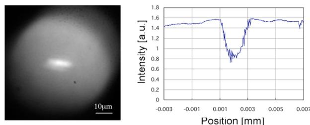
Fig.2 Blur-corrected image (latex particle of  $1\mu\text{m}$ ) with median filter observed at the Photon Factory.
