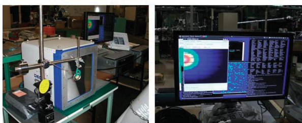
Figure 5 New pixel array X-ray detector. Commissioning of the detector (Pilatus 2M, Dectris) at the PF experimental hall using a calibration X-ray source.
