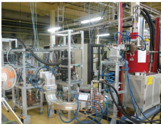
Figure 20 Coupler test stand with 300 kW klystron.
