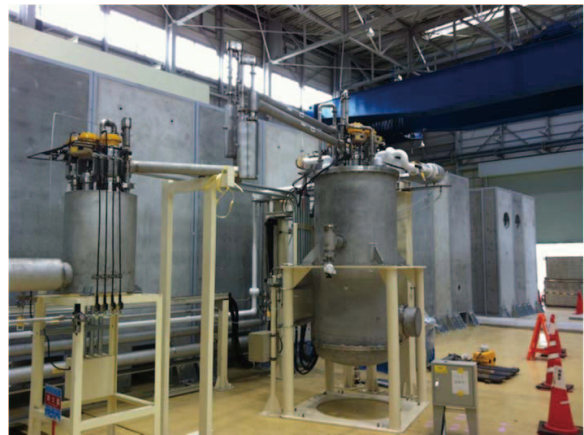
Figure 24 2K helium refrigerator cold box for injector linac under cold test.
