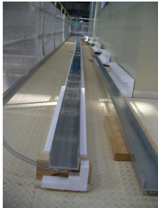
Figure 22 Cable shield for temperature regulation. It consists of an aluminum shield with water cooling channel and plastic thermal insulator.
