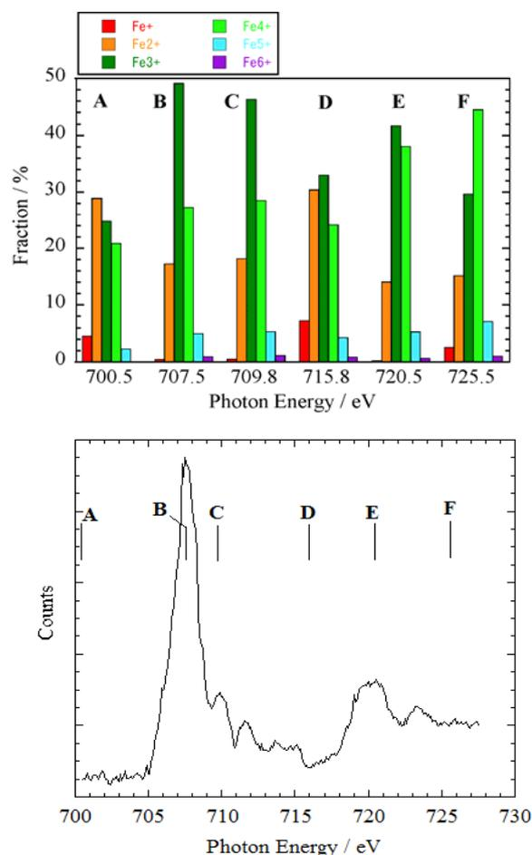
**Figure 1.** Top: Charge-state distribution at selected (A, B, ...) photon energies. Bottom: Total photoion-yield spectrum in the  $2p \rightarrow 3d$  excitation region.
