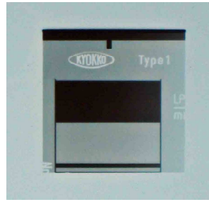
Fig.2a Image of Square Wave Chart Spatial Frequency : 0.0Lp/mm
