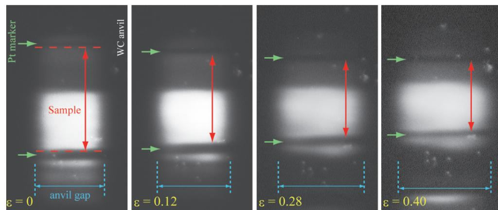
Figure 1: X-ray radiographs acquired before ( $\epsilon = 0$ ) and during the deformation ( $\epsilon =$  up to 0.40) at 1.7 GPa and 1370 K. Positions of platinum strain markers (black lines) are shown by green arrows. Blue and red double arrows represent the anvil gap and the range of sample, respectively.  $\epsilon$  represents the sample strain.
