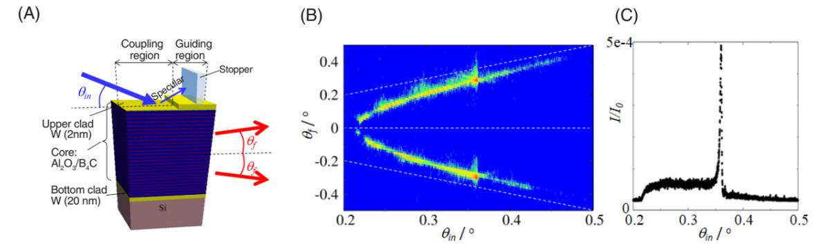
Figure 2: (A) The structure of the waveguide and the measurement geometry, (B) dependence of the far-field pattern on the incident angle  $\theta_{in}$ , (C) dependence of the normalized X-ray intensity on  $\theta_{in}$ .
