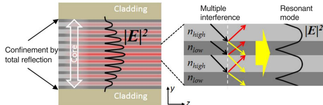
Figure 1: The concept of the periodicity-resonant X-ray waveguide.
