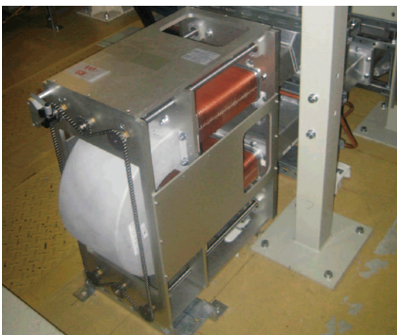
Figure 10: Variable waveguide phase shifter for adjusting the cavity input phase.
