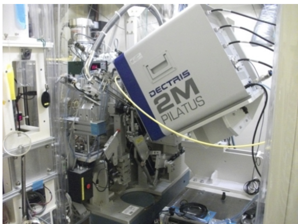
Figure 4: A newly installed Pilatus 2M detector at BL-1A.
