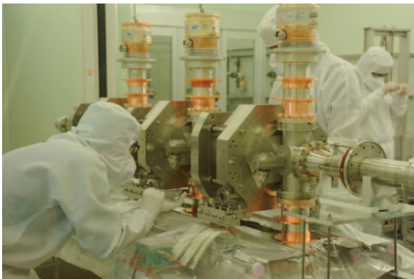
Figure 4: The assembly of the super conducting cavities for injector in a clean room.
