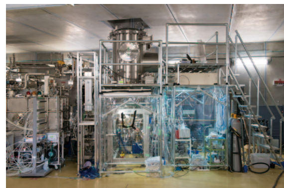
Figure 3: Photograph of the injector part of the cERL with 500-kV DC electron gun and super conducting cavity for injector.
