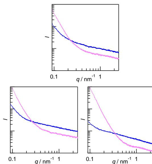
Figure 1. SAXS profiles of PEG/PNIPAm binary gels in the swollen state. The blue and red lines correspond to 20 and 40 °C, respectively. (Top) nonporous gel, (Bottom left) small-pore gel, and (Bottom right) large-pore gel.
