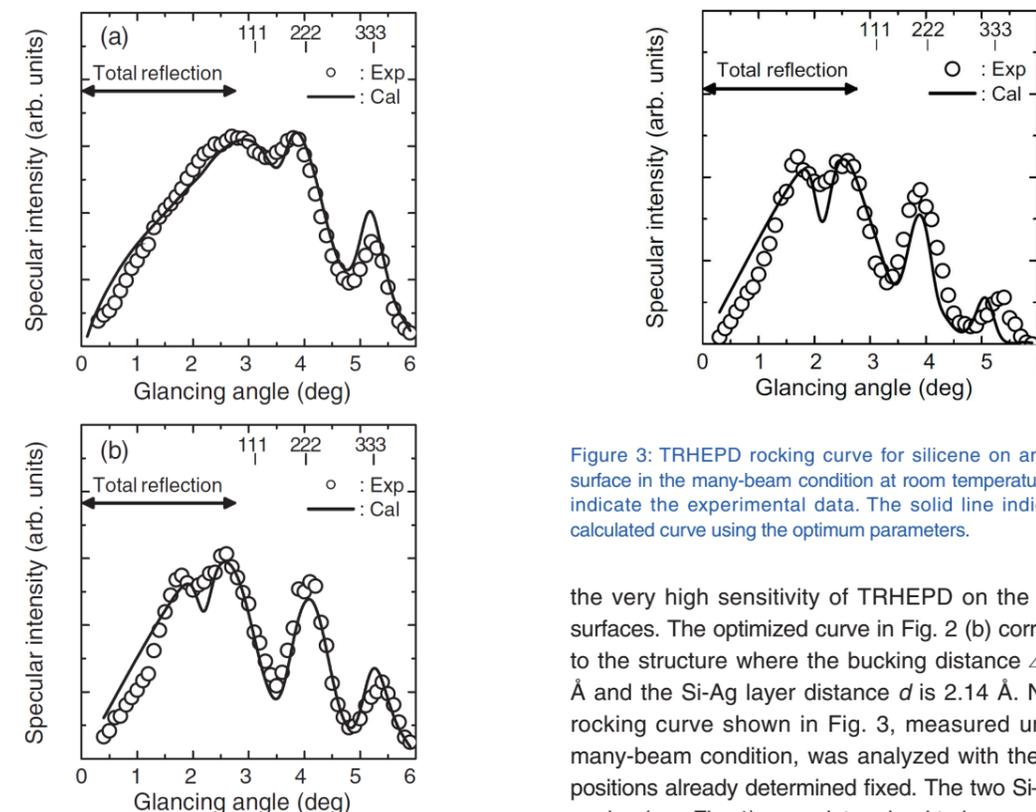
Figure 2: TRHEPD rocking curves for (a) Ag(111)-(1×1) surface before the Si deposition and (b) silicene on an Ag(111) surface in the one-beam condition at room temperature. Circles are the experimental data. Solid curves indicate the results calculated with the optimum values for the adjustable parameters.
