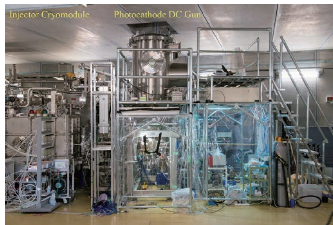
Figure 1: Photograph of a DC gun and cryomodule for injector cavities in a compact ERL injector.
