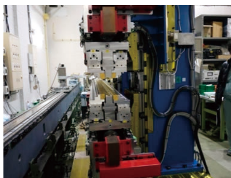
Figure 6: U#02-2 during the magnetic adjustment.
