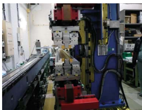
Figure 6: U#02-2 during the magnetic adjustment.
