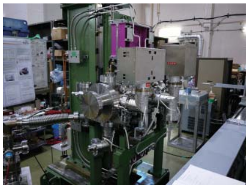
Figure 4: SGU#15 during vacuum commissioning.
