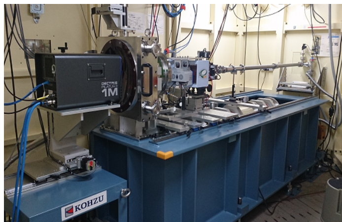
Figure 8: New experimental stage and detector, PILATUS3 1M at BL-6A.
