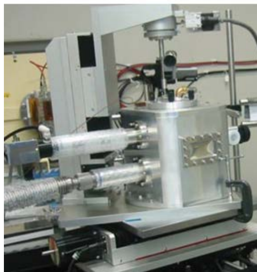
Fig. 1: Custom temperature-controlled chamber installed in the diffraction enhanced imaging (DEI) system.
