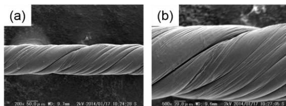
Fig.2 SEM images of twisted CNT yarn at twist number of  $3059 \text{ turns m}^{-1}$  observed at magnifications of (a)  $200\times$  and (b)  $500\times$ .
