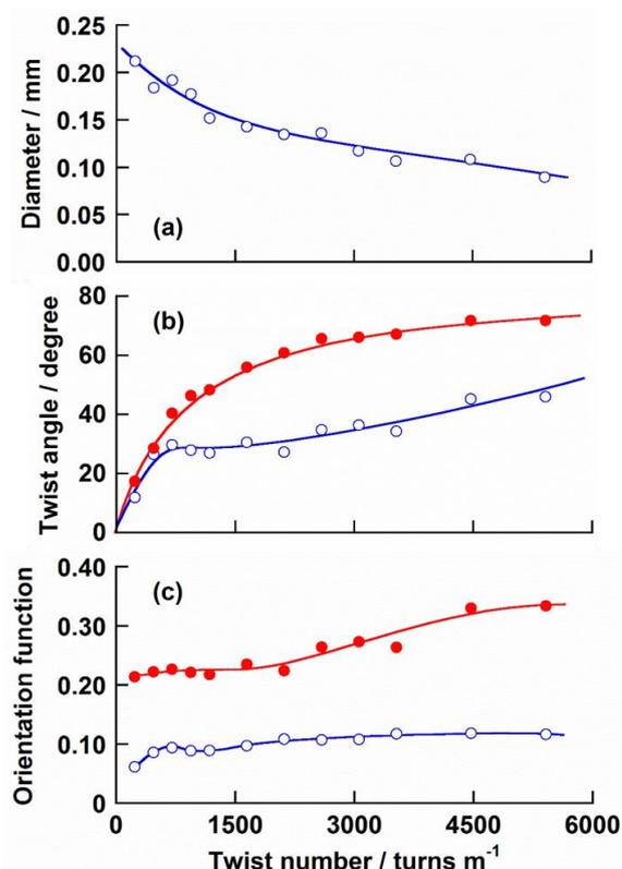
Fig.1 (○) Measured and (●) predicted values of (a) yarn diameter, (b) twist angle of CNT mat on yarn surface and (c) Hermans orientation function of CNTs versus twist number.
