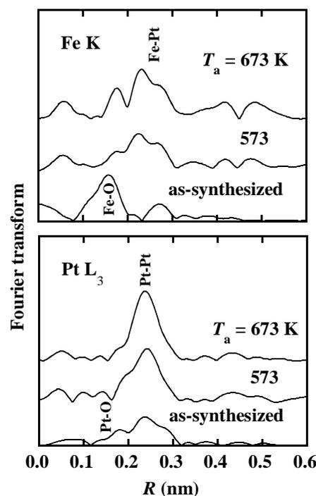
Fig. 1: Radial structure function around Fe and Pt atoms of the FePt nanoparticles synthesized at 383 K and those heat-treated at  $T_a = 573$  and 673 K.
