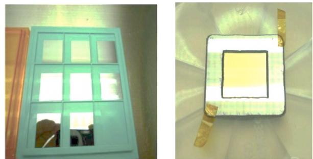
Fig. 1: The picture of test samples of mirrors (left) and a beam splitter (right).
