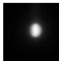
FIG.2. Measured image (64×64 pixels) of secondary diffracted beam ( E = 30 keV) through 1-mm-diameter-tungsten pin hole from Si(220) tandem crystal monochromator at the BL-14C. The fundamentally diffracted beam is absorbed with a 10-mm-thickness-aluminum filter. As additional absorber, 8-mm-thickness-aluminum filter is used to prevent from the over flow of the CCD. The maximum signal of the CCD is maintained to be less than half of the dynamic range.
