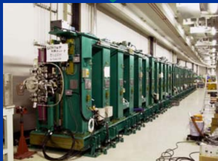
27 m-long in-vacuum undulator
