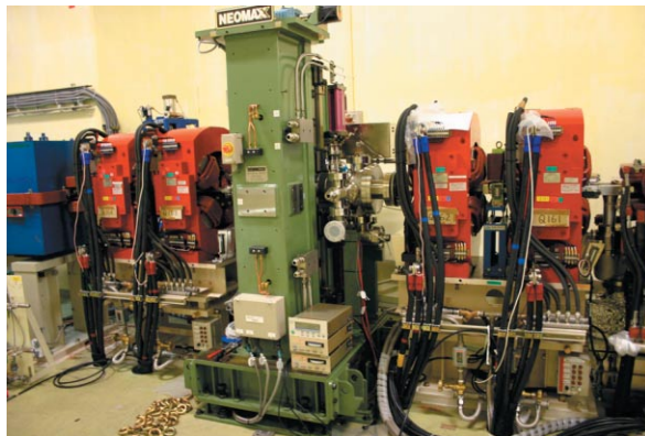
Figure 13 Short period undulator #17 installed in the ring.
