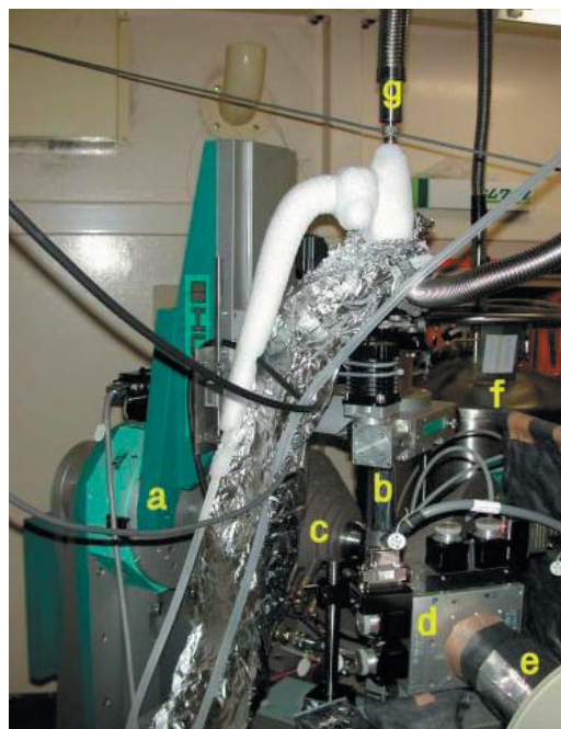
Figure 16 Experimental setup of the white X-ray magnetic diffraction of \text{YTiO}_3 : a, five-circles diffractometer; b, refrigerator of liquid He-flowing type to keep the temperature of the specimen at 5 K; c, electromagnet producing 0.3 tesla at a gap length of 50 mm; d, slit for receiving diffraction beam and minimizing fluorescent radiation from the specimen; e, pure Ge solid state detector; f, vessel of liquid He; g, transfer tube of liquid He.
