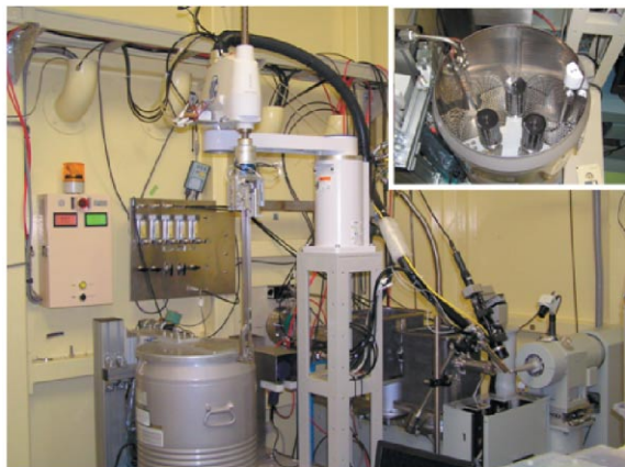
Figure 21 Overview of the sample exchange robot installed at AR-NW12A beamline. The inset shows an inside view of the Dewar in which three SSRL cassettes are held in place.
