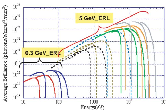
It is possible to cover the energy range from VUV to X-ray by using 5GeV ERL and 0.3GeV ERL.
