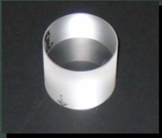
Sample photograph (30mm in diameter and 30mm thickness.)
