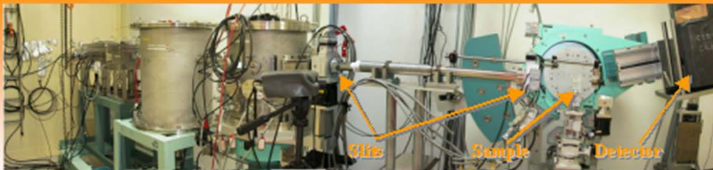
Experimental system (BL28B2 at SPring-8)
