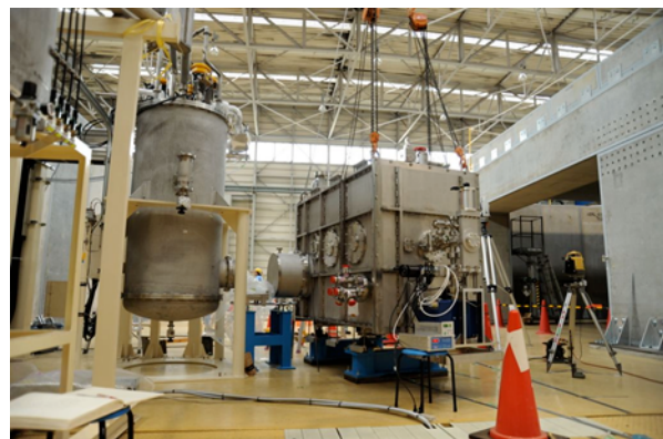
Fig. 2: Installation of the super conduction cavity for injector in the compact ERL at July of 2017
