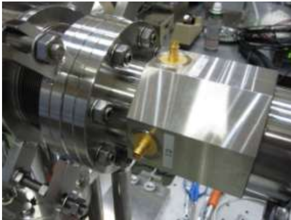
Stripline BPM with glass-type feedthrough
