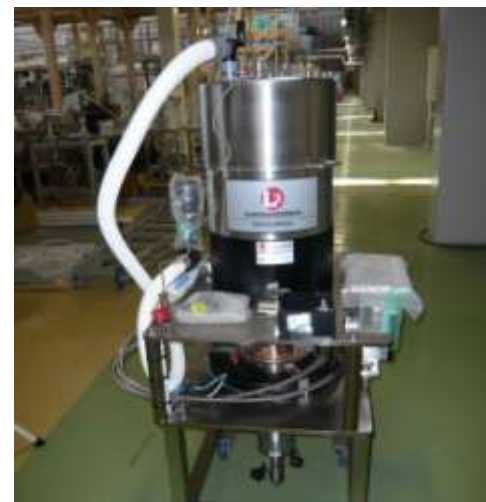
20kW CW IOT for buncher
