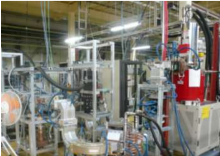
300kW CW Klystron for injector SCC
