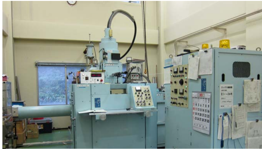
The electron-beam welding machine used for annealing of the moderator
