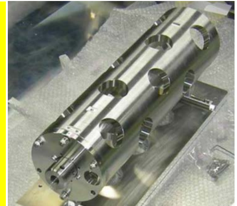
Pulse stacking cavity L_{cav} = 420 mm
