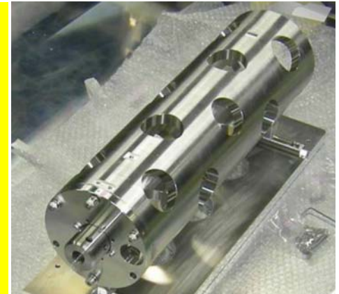
Pulse stacking cavity L_{cav} = 420 mm
