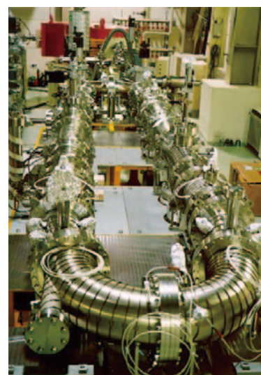
Electrostatic ion storage ring (Biomolecular ions such as DNA are stored as they are circulated within an accelerator ring, and the electron capture dissociation process of biomolecules is studied.)
