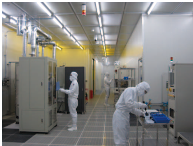
Clean room for producing SiC power device prototype
