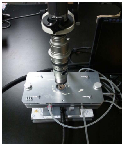
Figure 1 Photo of our new developed microscope, High Speed Polarized Optical Microscope (HSPOM).
