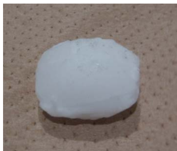
Figure 2 Natural gas hydrate pellet at 253 K under atmospheric pressure.
