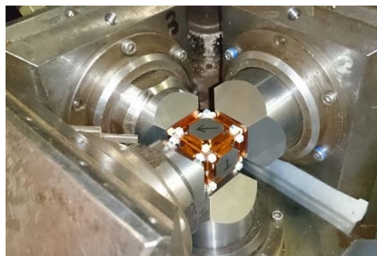
Figure 6 First anvils and second anvils.
