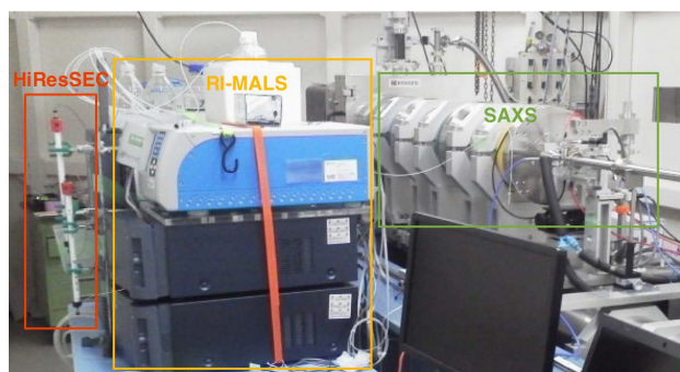
Figure 4 HiRes SEC-SAXS system conducted at BL-15A2 beamline of Photon Factory.
