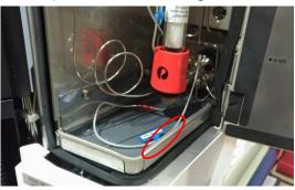
After the connection of column, set the flow rate and start the column equilibration.
