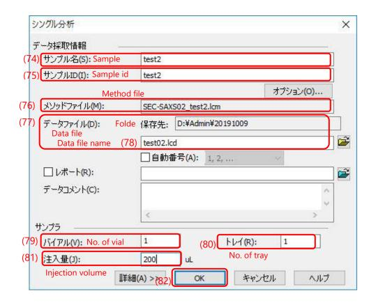
3-25 Click OK bottom (82) in the single analysis window to start injection of HPLC.
