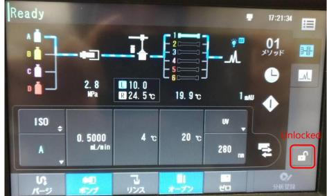
Touch the solvent bottle icon (3) on 分析メイン画面 [Analysis Main Screen] of the front LCD panel to open ポンプタブ [Pump tab] on [Parameter screen], and check the following parameters.
