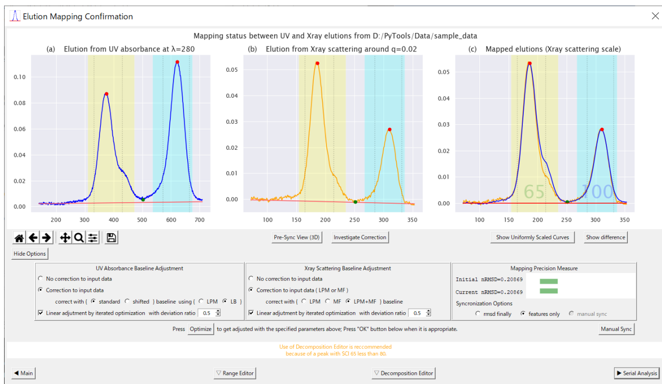
Fig. 6-9 Another Mapping Example where the Deviation is significant between the mapped Curves
