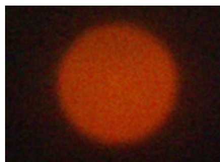
Fig. 3 : Fluorescence of the scintillator when it is irradiated with 140eV SX light passing through a \phi 20 \mu\text{m} pinhole positioned in front of it.
