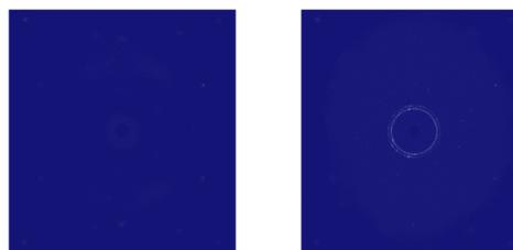
Fig. 2 XRD patterns for liquid state (left) and solid state (right) of lubricating oil
