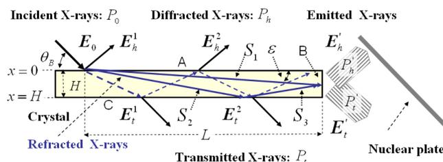
Fig. 1. Schematic diagram of Bragg-(Bragg)<sup>m</sup>-Laue case with  $m=0$  and 1.  $L$  is the distance from the incident point to the side surface B.
