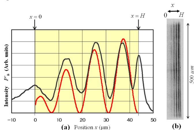
Fig. 2. Interference fringes of  $P_h'$ . (a) Intensity distributions and (b) Photograph of  $P_h'$ .  $L=891$   $\mu\text{m}$ .
