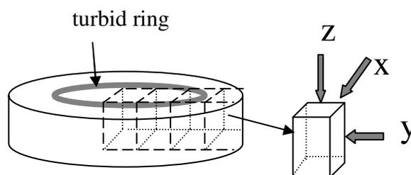
Figure 1. Illustration of the sample geometry. The scattering profiles were observed by irradiating X-rays from the indicated directions.
