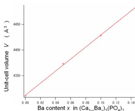
Fig.1. Compositional dependence of unit-cell volume of  $\alpha$ -TCP,  $(\text{Ca}_{1-x}\text{Ba}_x)_3(\text{PO}_4)_2$ .
