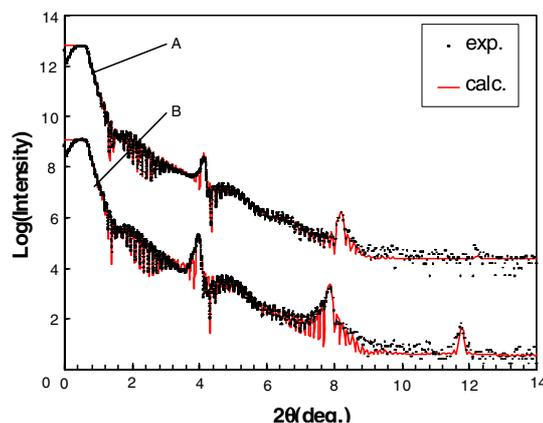
**Figure 1.** Measured (dot) and calculated (line) X-ray reflection intensity for sample A and B.
