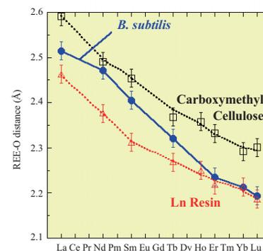
Figure 3 Average REE-O bond lengths of REE adsorbed on reference materials (carboxymethyl cellulose and Ln resin) and *B. subtilis*.
