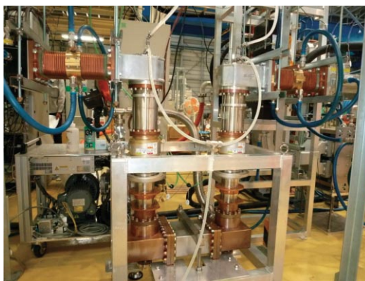
Figure 13 A high-power test stand for input couplers at the ECH (left) and the data logged for RF power and vacuum pressure during RF conditioning (right).
