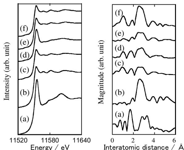
Figure 1 Pt L<sub>III</sub>-edge XANES spectra (left) and FT-EXAFS spectra (right) of (a) PtO<sub>2</sub>, (b) Pt foil, (c) Mw-Pt-TiO<sub>2</sub>, (d) PAD-Pt-TiO<sub>2</sub>, (e) EA-Pt-TiO<sub>2</sub> and (f) Imp-Pt-TiO<sub>2</sub>.
