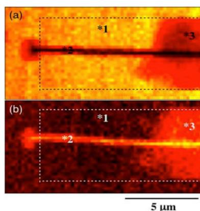
**Fig. 1.** Chemical images obtained by tuning binding energies for (a) Hf 4*f* and (b) Si 2*p* core-level photoemission spectra in poly-Si gate patterned samples.
